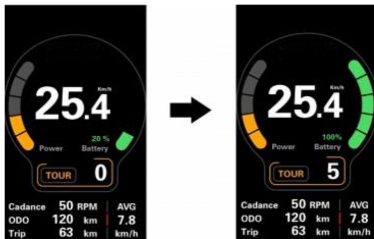
Battery SOC Indication Interface
